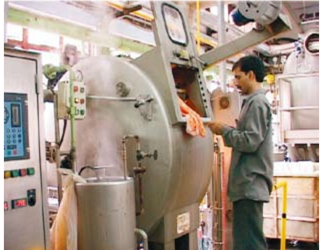
The fabric is dyed in large drums. Temperature increases and timings have to strictly follow the recipes of the dye manufacturer.
