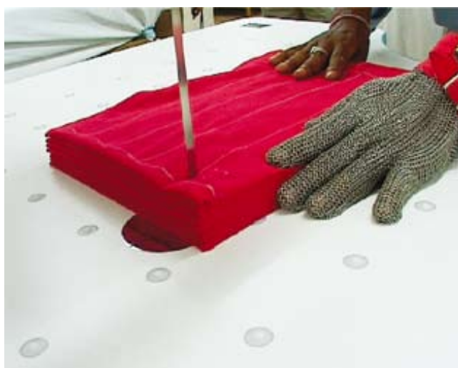
Then the whole bunch of cloth is cut together with this kind of 'sawing' machine
