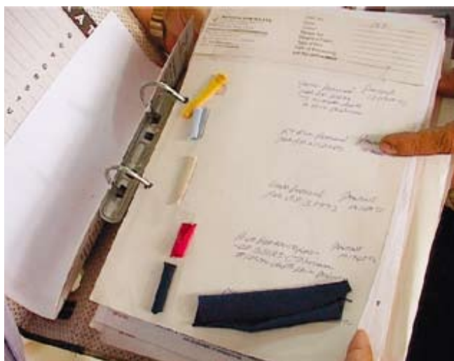
Samples of the colour tones are sent to Ciba Geigy, who provide a recipe to match the colour
