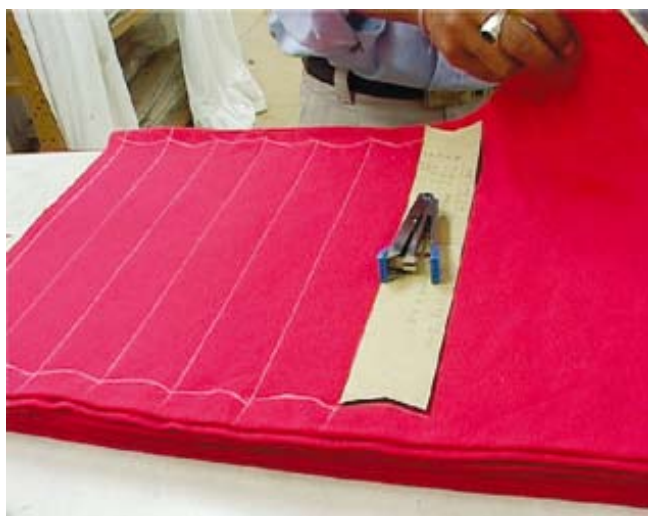
Depending on the cutting pattern, the different parts are marked with a white pen on the top cloth
